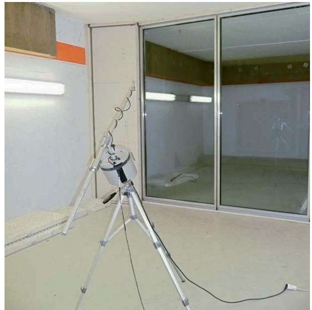
In our own certified echo chamber and wall test stand we test absorption properties and sound insulation.
