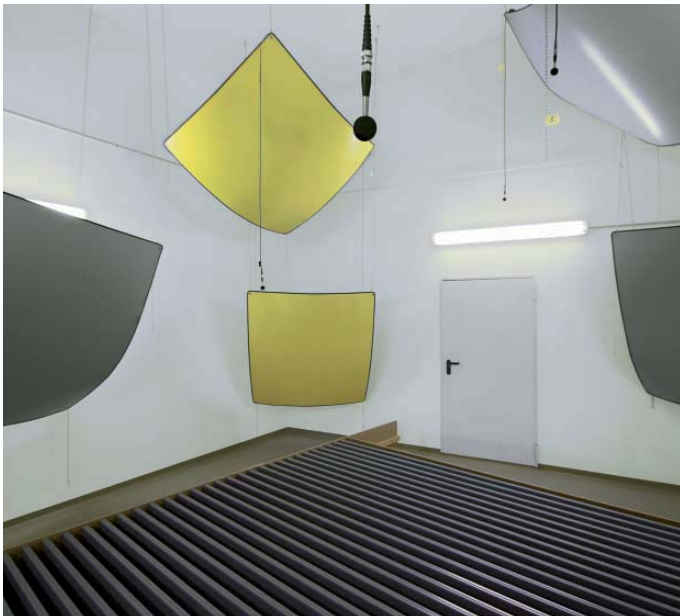
In our own certified echo chamber and wall test stand we test absorption properties and sound insulation.
